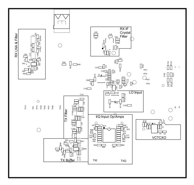
Figure 6 – PCB Layout: bottom
