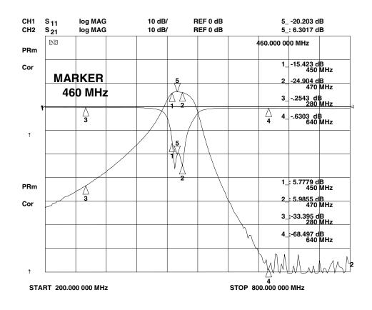
Figure 8 – Typical response of optional Tx filter + buffer.
