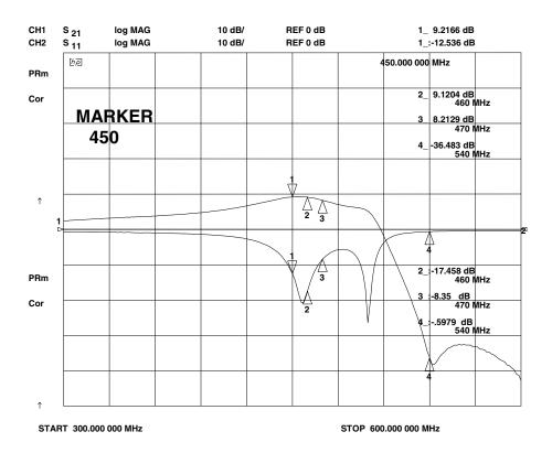
Figure 7 – Typical LNA  $S_{21}$  and  $S_{11}$  response
