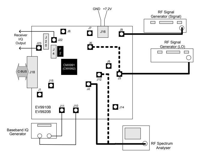
Figure 2 – Typical Evaluation Connections for EV9910B/EV9920B
