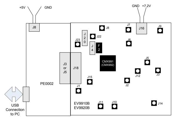
Figure 3 – EV9910B/EV9920B Connection to PC Using PE0002
