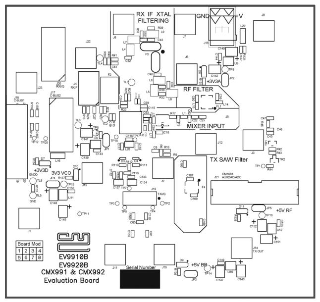
Figure 5 – PCB Layout: top
